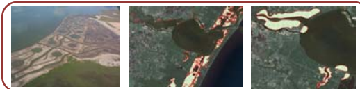
Figure 6: Bottom Friction and Surface Canopy parameters extracted from Wetlands databases and hypothetically generated in GIS. Spatially weighted formulation to calculate finite element node parameter. a) Database; b) Bottom Friction; c) Thiessen Polygon spatial averaging; d) Updated FE nodes
