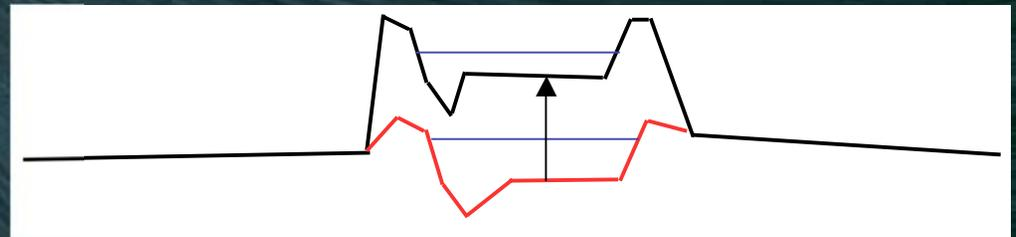
Stop-bank levees cause super-elevation of the channels above the surrounding floodplain.
