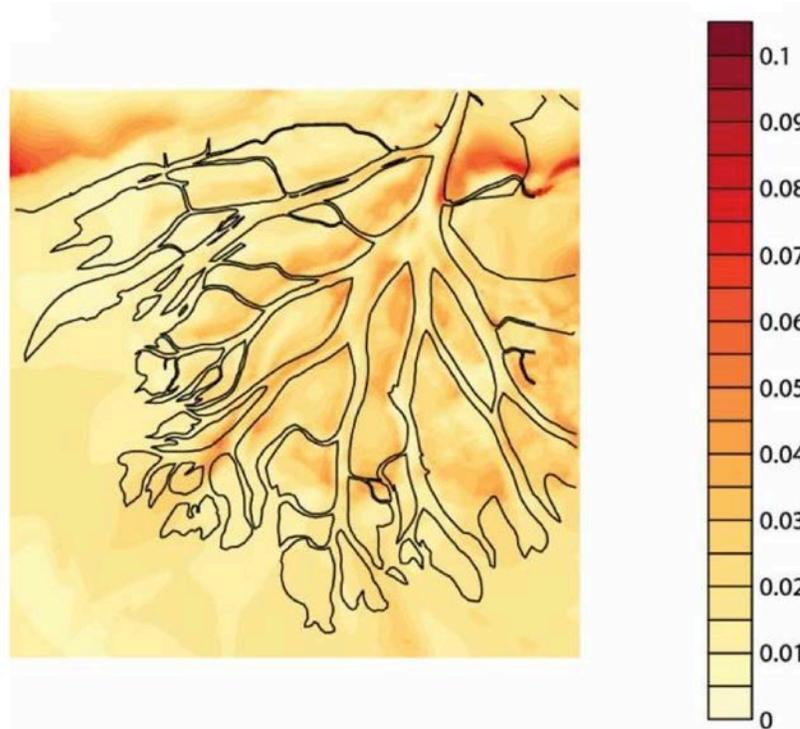
**Fig. 4.1** Spatial uncertainty of surface elevation, characterized by its standard deviation (meters), in the Wax Lake Delta in the aftermath of Hurricane Rita, from 81 Delft3D simulations. Excerpted from Fei Xing's PhD dissertation.
