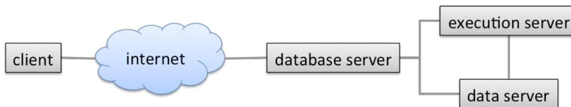
Figure 3.2. The relationship between the WMT client and the WMT servers.
