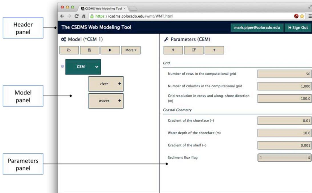
Figure 3.2 Example of the WMT client interface, with primary components highlighted.
